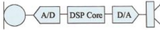
Fig. 1. Block schematic of a DSP hearing instrument with (l to r) microphone, A/D, DSP core, D/A and receiver.
